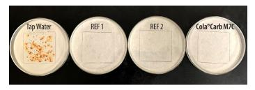
ASTM D4627: Soaked at room temperature during 24 hour study period
