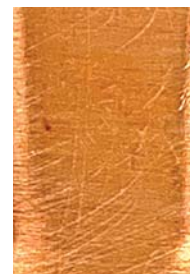
Copper with 2% KAT (6 hours @ 80°C)
