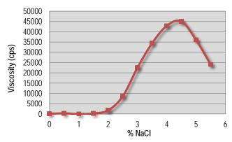
Salt curve test is performed with a blend of SLES-2 and Cola®Liquid BL, ratio of 5:1, diluted to 12.9% solids with water.
