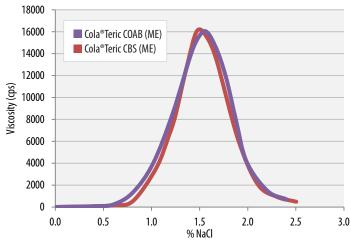
Test Solution: Water, SLS, SLES-2, Amphoteric + Cola®Liquid DC (ME) (all) 1.5 COAB (ME): 75/10/10/5; CBS: 74.8/10/10/3.7
